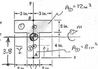
6. A horizontal force  $P = 20$  kips is applied to the beam shown. The maximum tensile stress in the beam is most nearly
