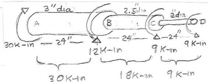
2. For the solid brass shaft shown,  $G = 17 \times 10^3$  ksi. The angle of rotation at section B is most nearly:
