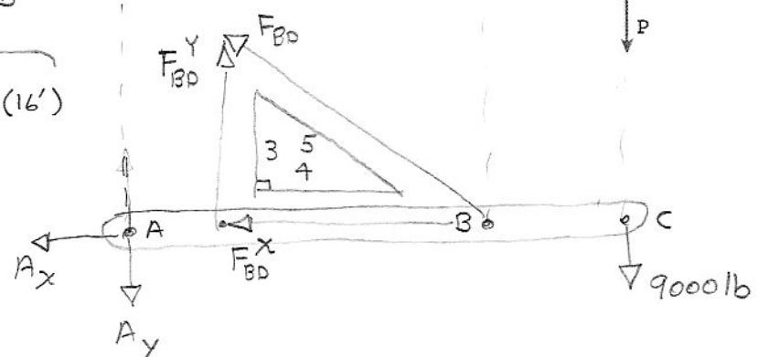
2. A flat bar is loaded as shown. The maximum stress in the member is most nearly
